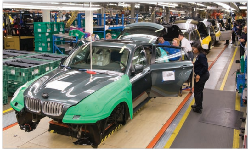
X models at the BMW plant undergo final visual inspection before receiving components such as power trains, transmissions, engines, and front and rear axles.
